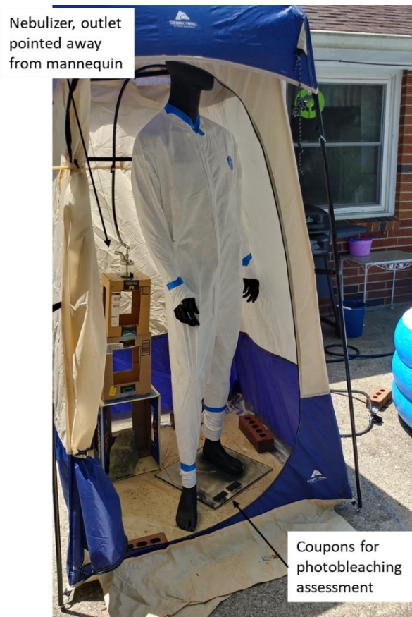
Figure 7. Exposure booth showing mannequin and nebulizer placement.
