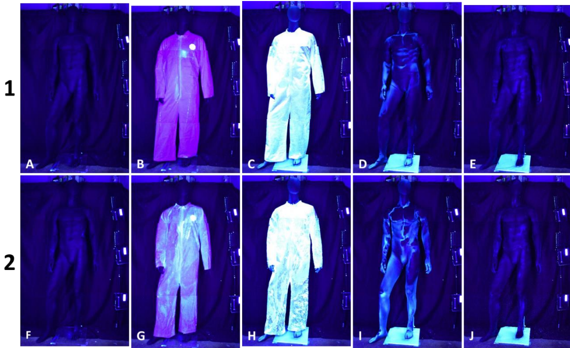
Figure 20. Representative images from 1) Trial with new suit and 2) Trial with re-used suit. From left to right images show the mannequin before exposure (A, B, F, G), the mannequin after exposure (C, D, H, I) and the mannequin after decontamination (E, J).
